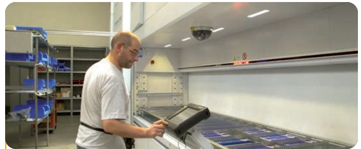
Put-to-light systems connected to WMS
