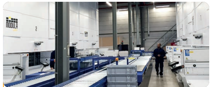
Integration with conveyors
